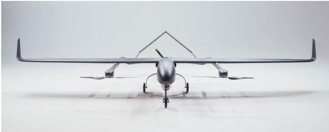
Figure 1.1 Hybrid VTOL Fixed-Wing UAV Produced by UKRSpecSystems
