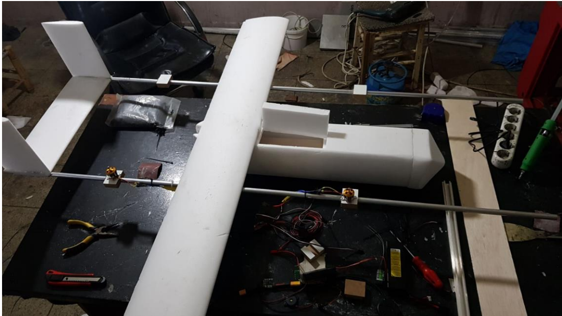
Figure 4.2. Wing and Tail Mounted on the Body
