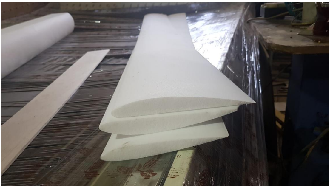
Figure 4.1. Fuselage and Airfoils Cut From XPS Foam
