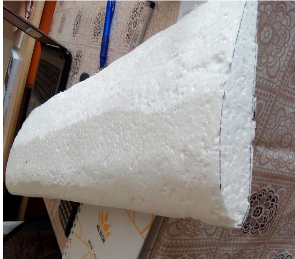
Figure 2.5. Failure NACA 4412 with EPS foam
