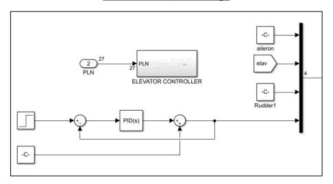
I've designed throttle controller for this mission. Throttle controller controls the velocity and elevator controller controls the altitude change. When I run this two controller together they manage their jobs to climb desired altitude. Elevator controller try to reach desired altitude and throttle controller provide required thrust to climb.
