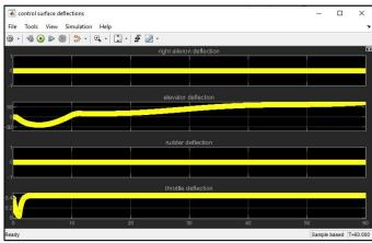
I can clearly see the deflections to reach desired altitude. I should mention that throttle defleciton is in the desired throttle range which is not provide higher than 0.2 mach
