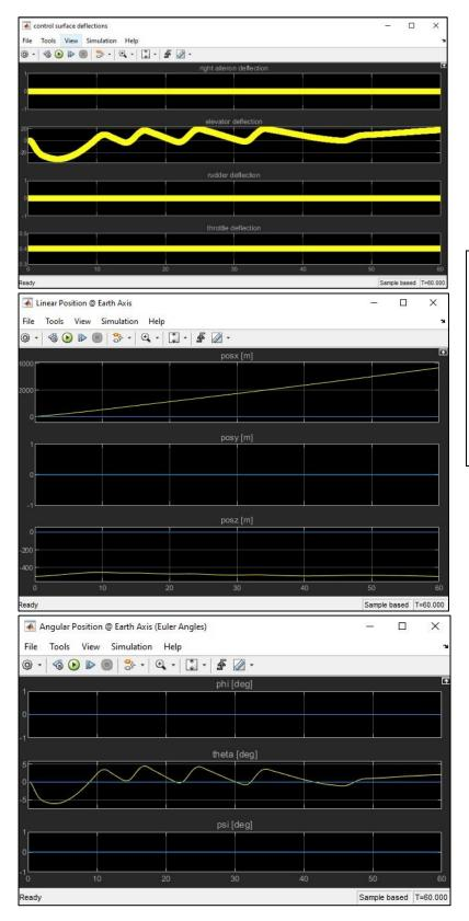
My controller changes the elevator deflection to fly initial altitude. As I see in the graphs posz stabilize after 7sec. Between 0 to 7 sec elevator controller sets its parameter for steady level flight to complete the mission Final results are very good for me.
