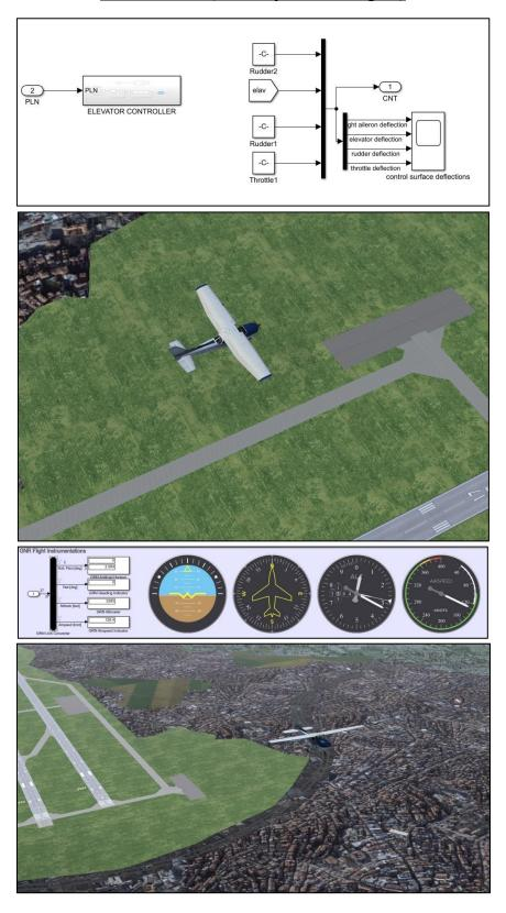
In this mission, I arranged an elevator surface controller to flight steady and horizontal. I designed this controller from matlab lightweight aircraft design also I've adjusted values, inputs and transfer functions for my aircraft which are suitable.
